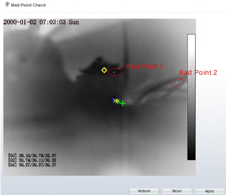
Figure 5-6 Bad Point Check
