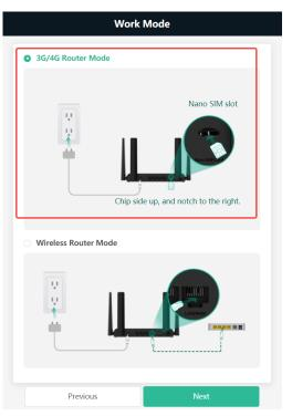
(2) Configure SIM card parameters: Generally, the system automatically populates the basic SIM card information. When an SIM card is available, you can access the Internet through the router. If the SIM card cannot be identified by the router, you need to enter values in the Profile, DPD Type, APN, Username, Password, and Authentication Type fields to enable the router to connect to the Internet. Keep the default settings unless otherwise specified, and click Next.
